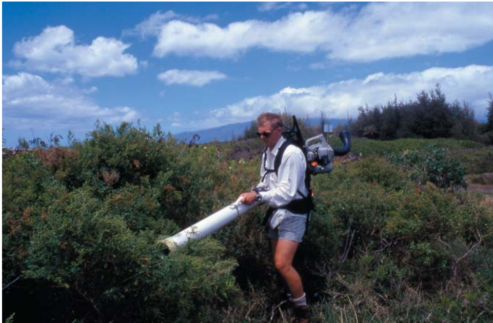
Figure 4.4. Gas aspirator device for mass sampling insects on vegetation (Photo: D. Preston).
