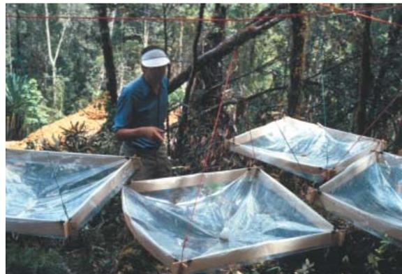
Figure 4.6. Simple, inexpensive collecting trays suspended under the forest canopy for collecting fogging samples (Photo: A. Allison).
