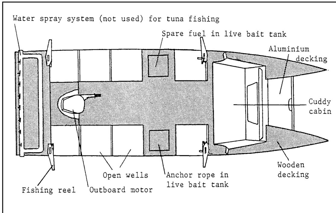
**Figure 3: Fishing arrangement of the Tautai Nioue**
